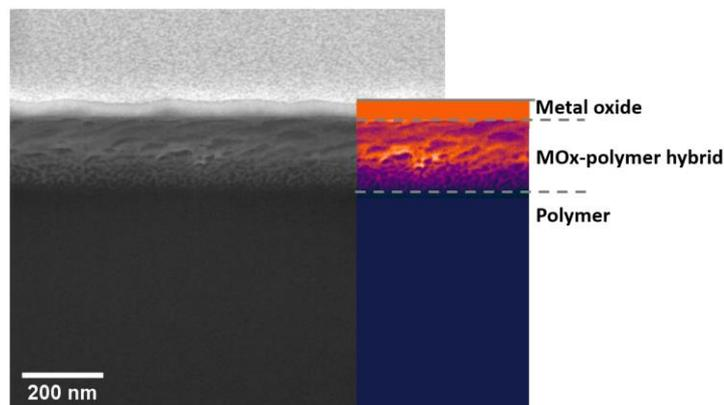
Fig.1. SEM micrograph of cross-section of PEN polymer modified with VPI of alumina oxide.
